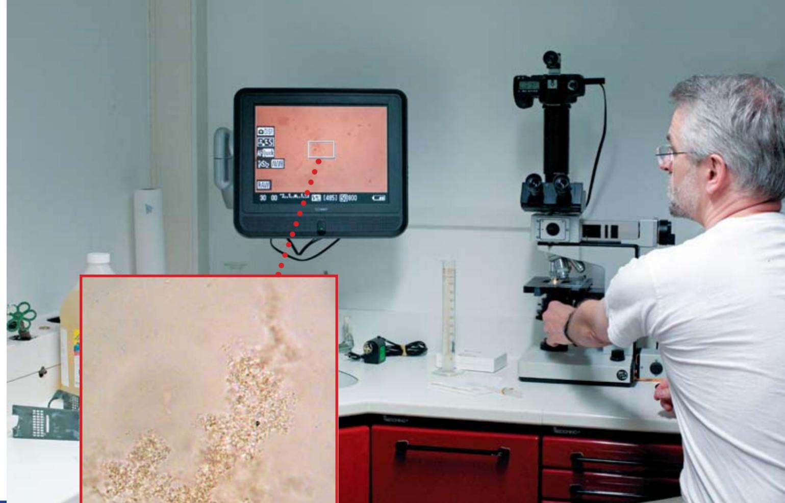
Lanthanum-phosphate flocculation under the microscope.
