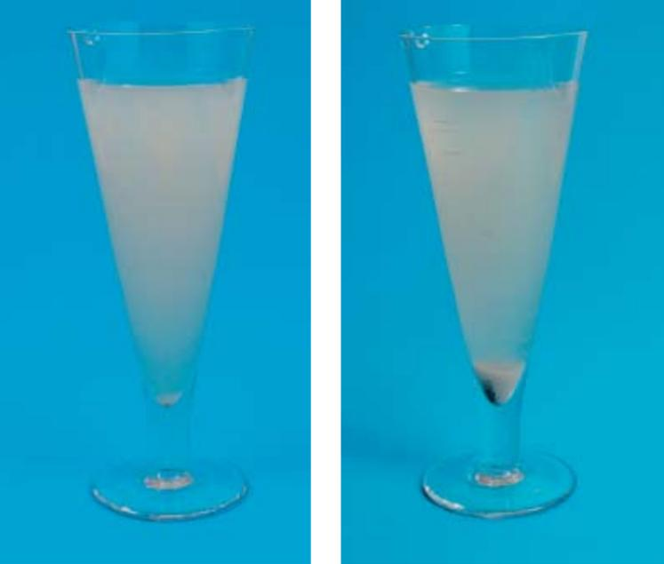
The filtrate was rinsed out of the floss into a glass – within a few minutes a significant layer of sediment had accumulated at the bottom.
