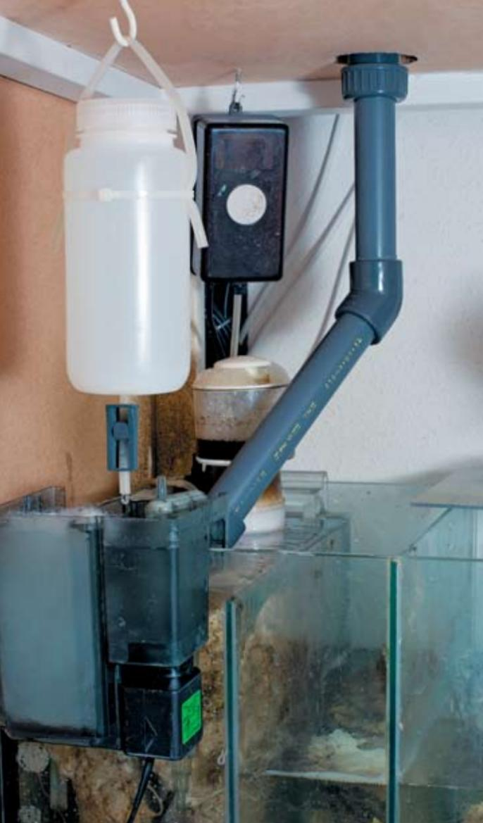
Experimental addition of diluted lanthanum chloride solution to an external filter filled with filter floss, feeding into a chamber of a filter tank containing a protein skimmer; within seconds of the beginning of the addition of lanthanum the skimmer overflowed. The drip rate was regulated using a dosing clamp, such as is used for medical infusion, on the feeder tube.
